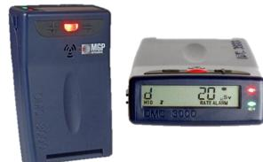
CERN Operational Dosimeter: DMC 3000 from Mirion
